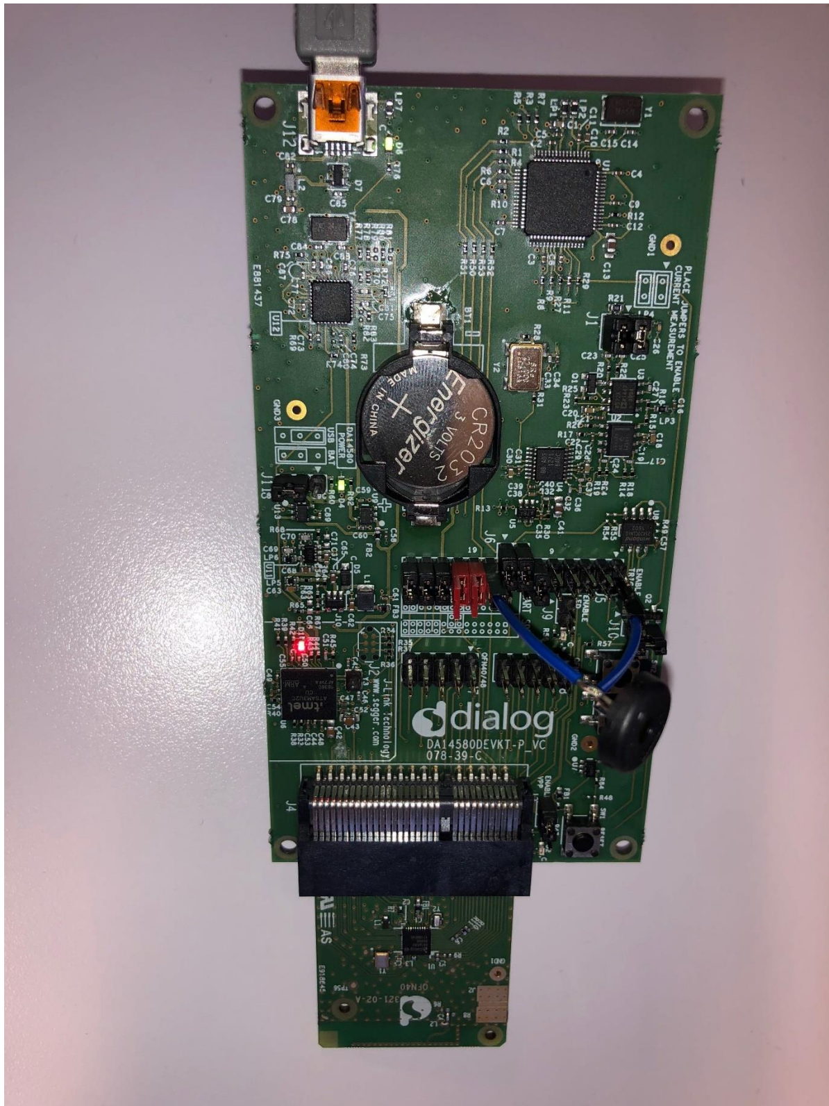
Picture of a Configured DA14585 Development Kit Pro:
