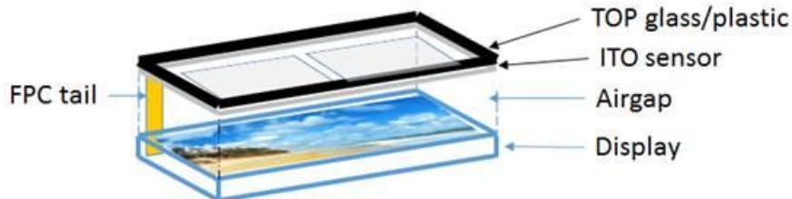
Figure 11: ITO placement underneath the top glass cover
