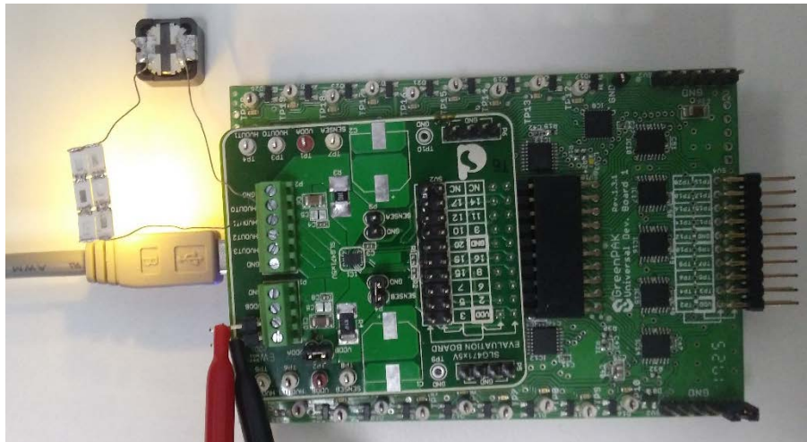
Figure 4: Warm LEDs On, Cold LEDs Off
