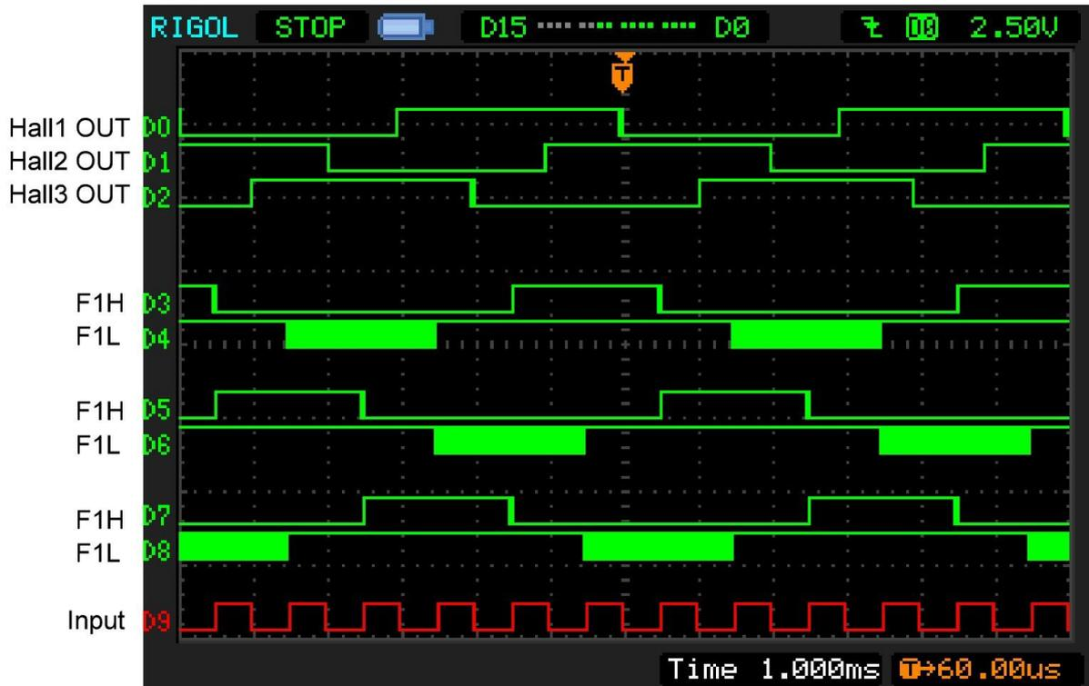
Figure 6: BLDC Motor Operation Scope Shot
