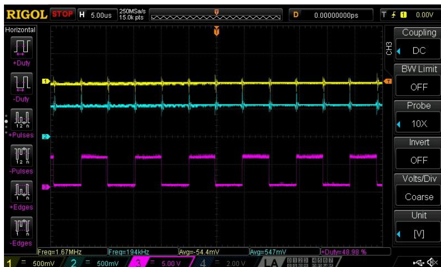
Figure 12: 50% Output Duty Cycle, ANALOG_IN \approx 550 mV
