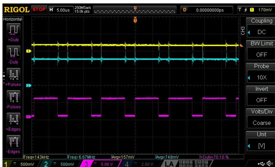
Figure 11: 70% Output Duty Cycle, ANALOG_IN ≈ 700 mV
