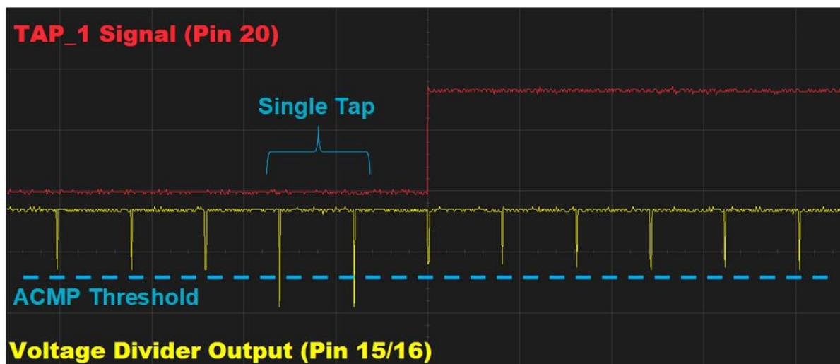
Figure 7: Single-Press Signal
