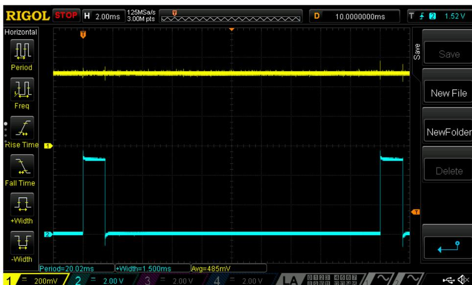
Figure 7: PWM Signal for Center Servo Position
