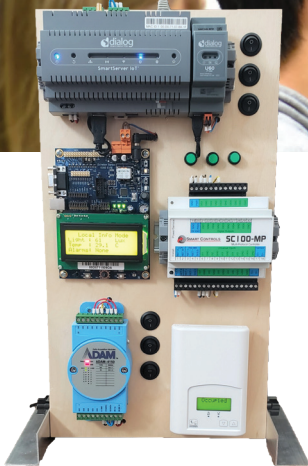
Pre-assembled panel with SmartServer IoT and typical industrial devices ships in a travel case
