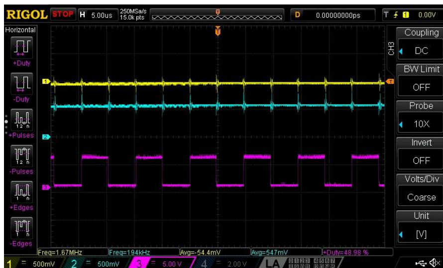
Figure 12: 50% Output Duty Cycle, ANALOG_IN ≈ 550 mV
