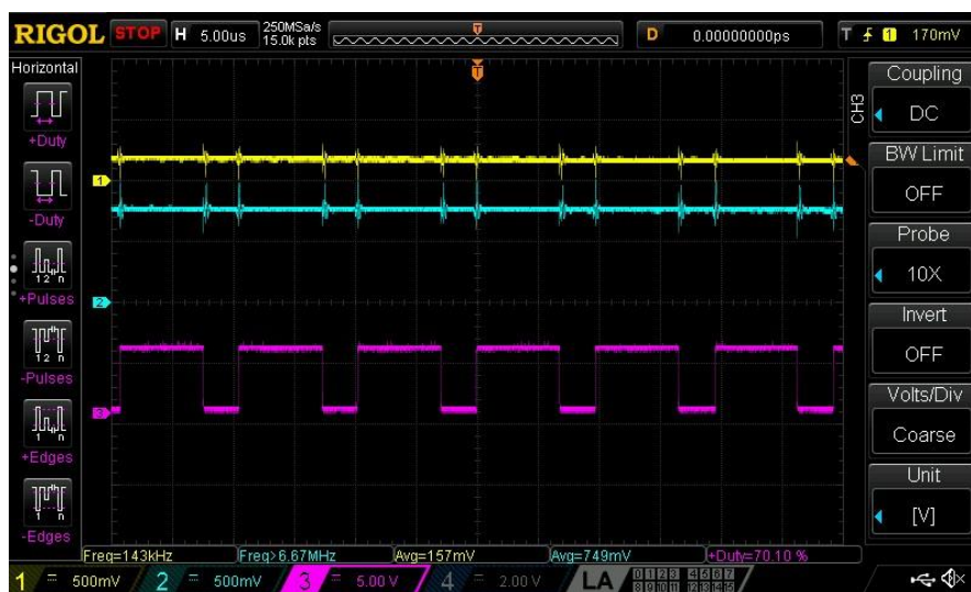
Figure 11: 70% Output Duty Cycle, ANALOG_IN ≈ 700 mV
