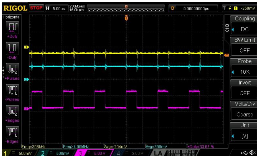
Figure 13: 30% Output Duty Cycle, ANALOG_IN ≈ 400 mV
